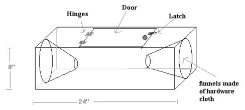
Figure 3. Funnel trap design made with quarter inch plywood.
